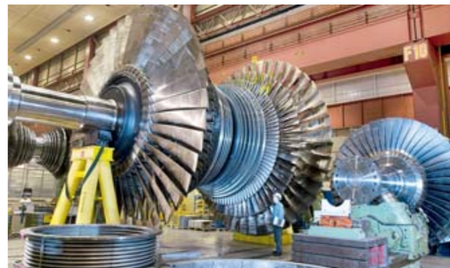
Twice as big as an Airbus A380 turbine, the steam-turbine rotor being manufactured in Siemens' Mülheim an der Ruhr factory is the biggest and heaviest in the world.
