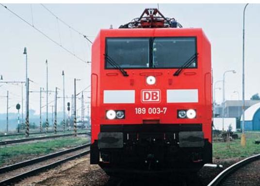
Siemens has developed a special headlight for the new BR 189 Europa Locomotive. The headlight consists of over 400 LEDs that can produce a wide variety of patterns.
