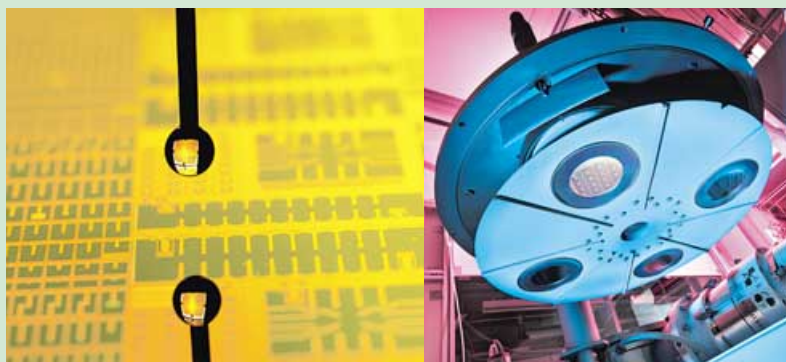
A micropipette (left) deposits a nano-liter of a biomolecular solution on a test sensor array. A sputter system for the piezo layer of the sensor (right).
